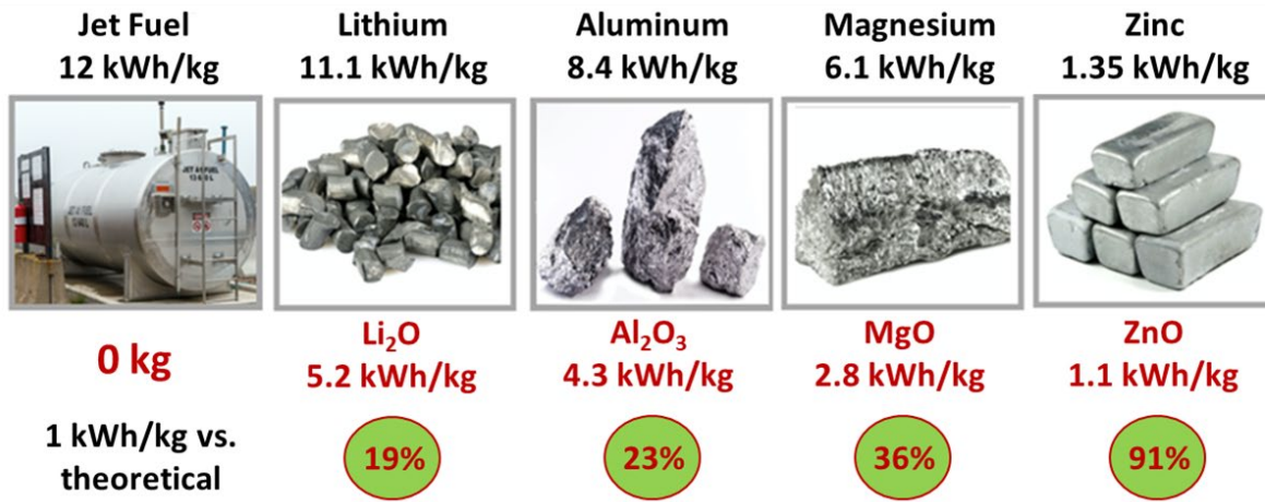
Figure 3. Theoretical energy densities of metals as fuels together with the corresponding oxides.
